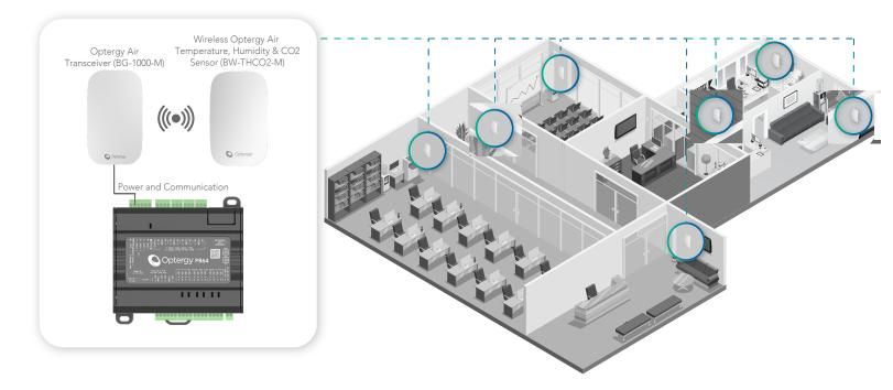
The Optergy Air BW-THCO2-M sensor pairs with the Optergy Air Transceiver (BG-1000-M). Up to seven (7) Optergy Air BW-THCO2-M sensors can be connected to one Optergy Air Transceiver (BG-1000-M).
